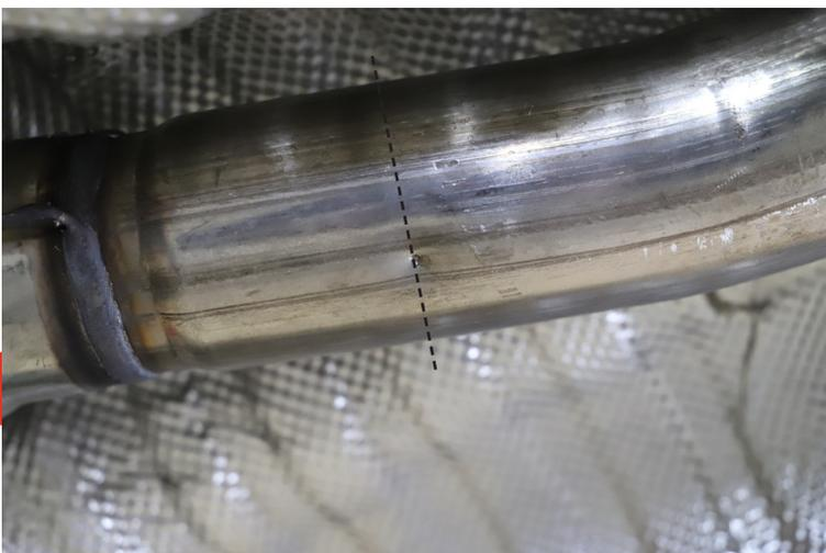
To make it easier to cut the exhaust we recommend removing it from the car. Find the indent just before the resonator to mark out the cutting line. Cut along the line and de-bur the edges. Re-fit the original GPF and fit the Scorpion GPF-back following the line diagram on the first page.
